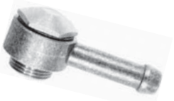
Fuel Inlet Swivel Fitting Hose: 5/16" 9/16-24 Thd. SP-25 (26-25)
