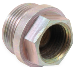
H15-96 Fuel inlet fitting (3/8 tube 7/8-20 OD thread 5/8-18 ID thread) "Allows 3/4 wrench to be used on fitting."
